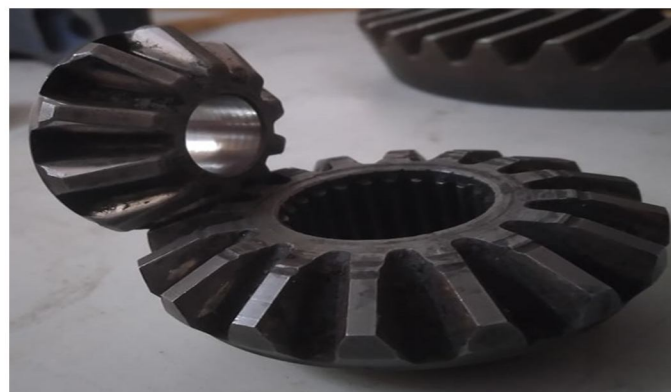
Fig4: Straight Bevel Gear
