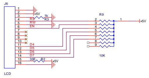
Schematics of LCD Interfacing
