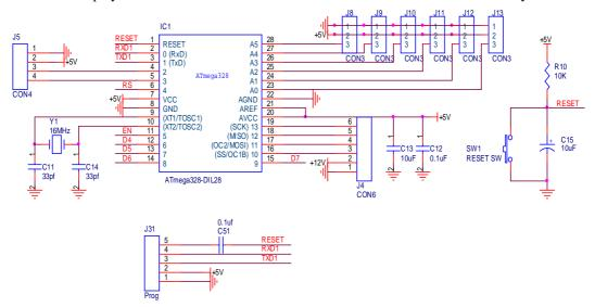
Schematics of Arduino Interfacing
