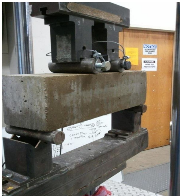
Fig. 8 Experimental setup for testing of beams
