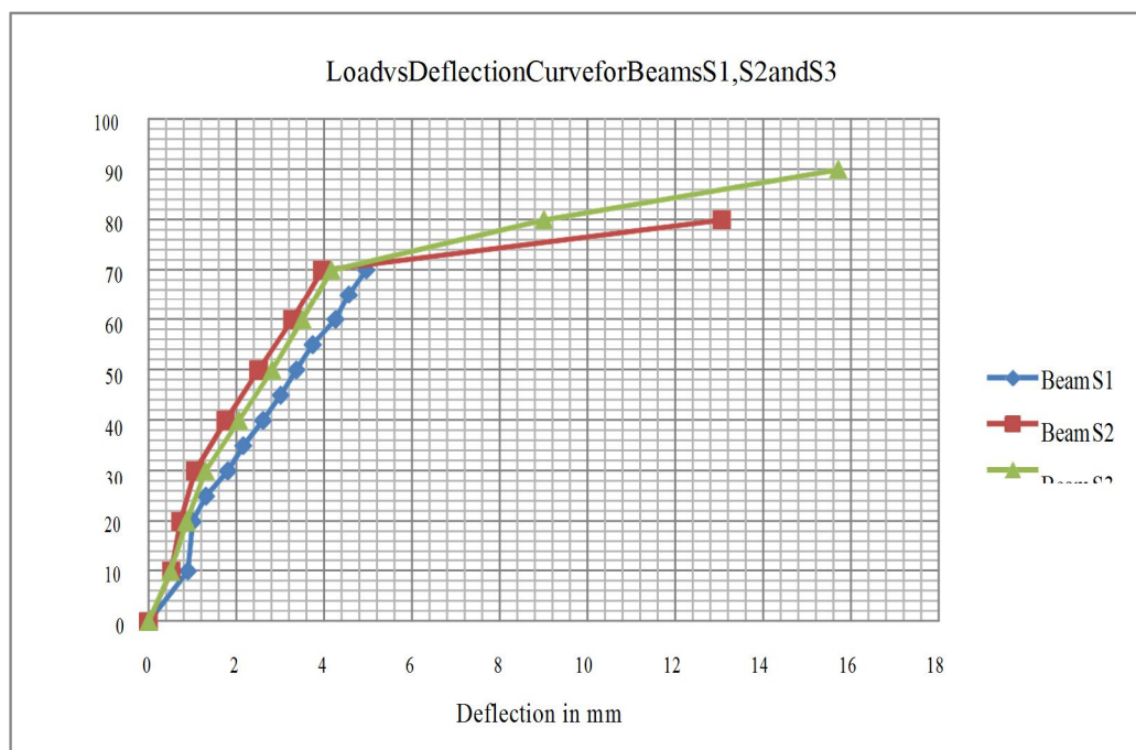
Fig. 10 Load vs Deflection Curves for Beams S1, S2 and S3.
