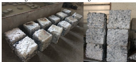
Fig 3.1 cubes after removing from acid tank
