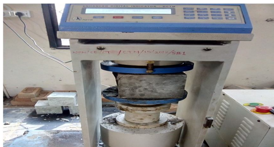
Fig no. 4.testing of cube
