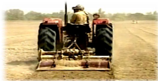
Fig: 2(d) Soil Pulverization by Rotavator Operation
