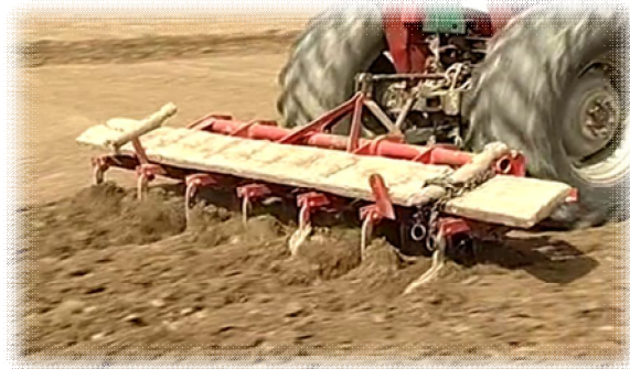
Fig: 2(c) Soil Pulverization by Cultivator Operation
