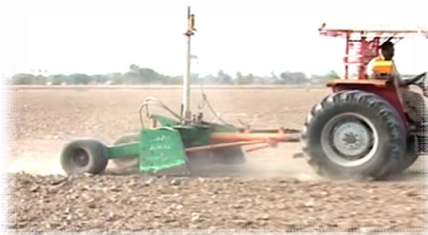
Fig: 2(e) Laser Land Leveling Operation
