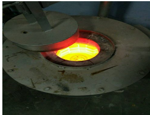
Fig. 8 Melting in Stir casting process
