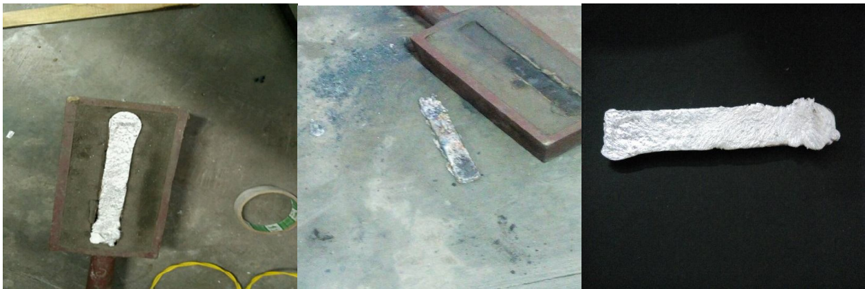
Fig. 9 Solidification of composite into the mould
