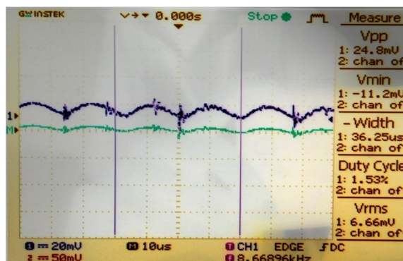
Fig 4.4 Inverter Neutral Voltage
