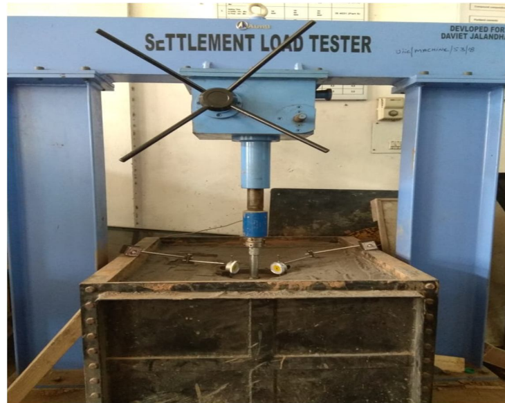
Fig. 3 Model tank including loading plate and dial gauges
