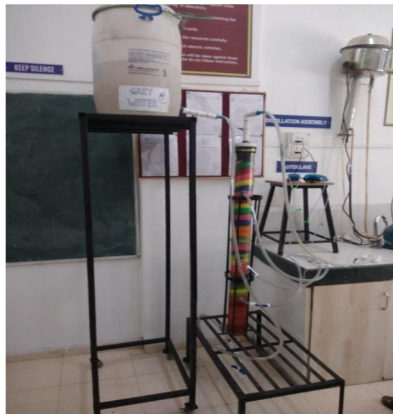
Fig 3 upflow packed bed aerated reactor actual setup
