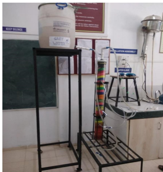
Fig 3 upflow packed bed aerated reactor actual setup
