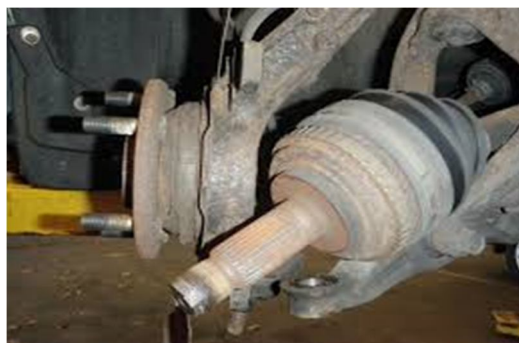
Fig :- IV b )Front Axle failure
