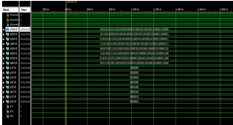
Fig15: Simulation for (72,64) Multi-bit Correction
