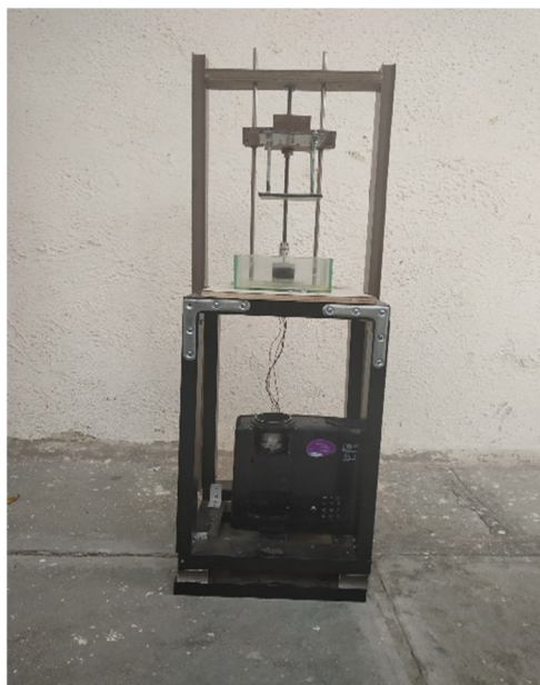
Fig.5 Final setup of our DLP 3D printer
