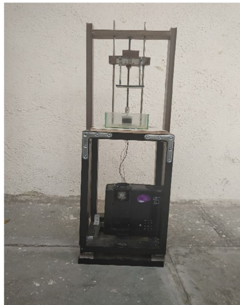
Fig.5 Final setup of our DLP 3D printer
