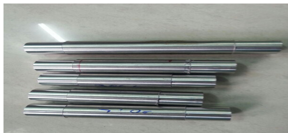
Fig 5.1 work piece material after turning
