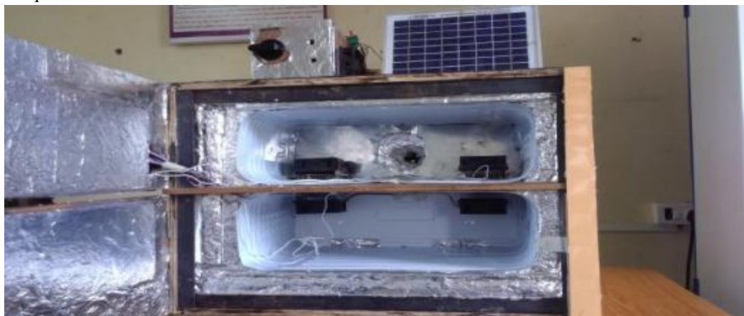
Figure 7. Designed Thermo-electric Heating & Cooling system.
