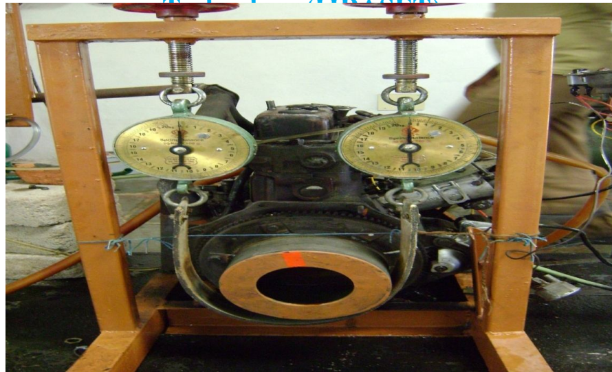
Fig 7. Experimental loading set up of 20 hp diesel engine with mechanical loading
