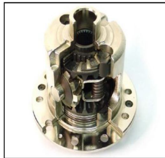
Fig 4: Clutch plate limited slip differential
