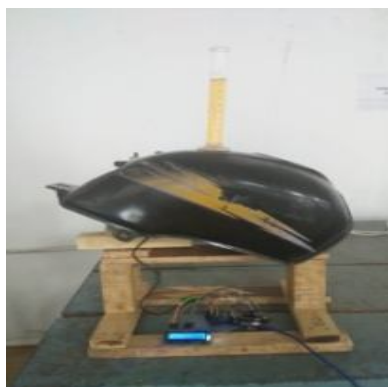
Fig.6 100ml of petrol filled in flask
