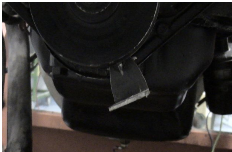
Figure 9. Setting a reference & triggering signal for cylinder #1
