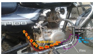
Fig. 3.1 Air Preheater installation on vehicle
