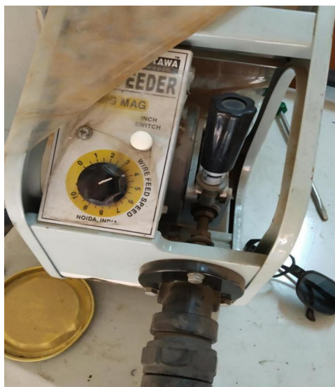
Figure-1: Experimental Setup of MIG welding machine
