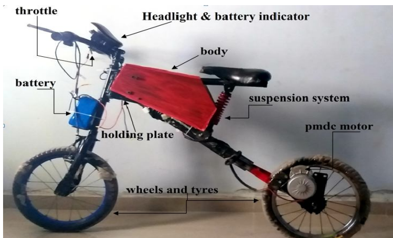
Figure1: key components of Foldable electric bike.
