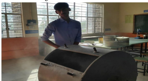
Figure 12 Los Angeles Abrasion test
