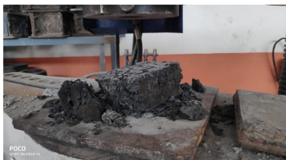
Fig. Compressive Test on Paving Block on UTM
