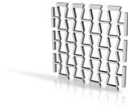
Fig. 6. Bow-tie network of auxetic materials
