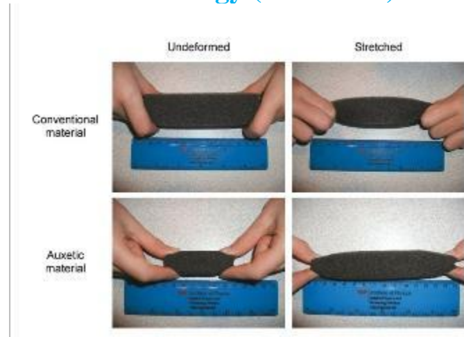
Fig. 2. An auxetic material increases in thickness under tension.
