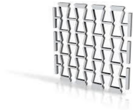
Fig. 6. Bow-tie network of auxetic materials
