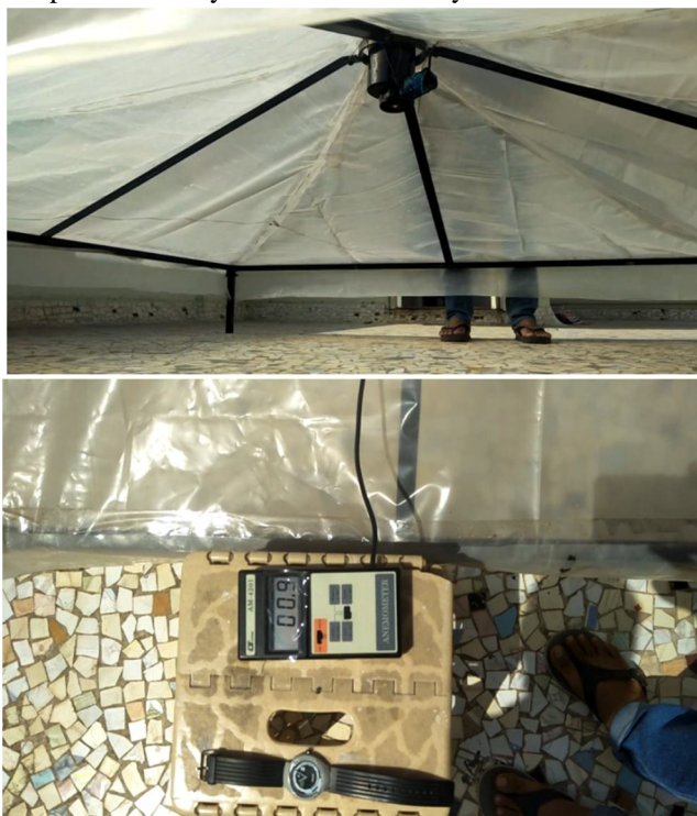
Fig. 2 Measuring velocity of air-flow with anemometer
