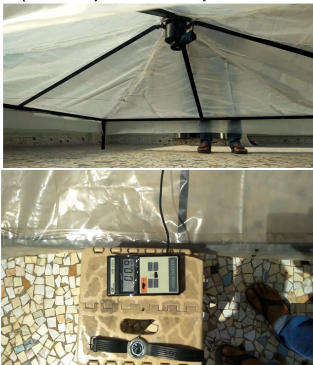
Fig. 2 Measuring velocity of air-flow with anemometer
