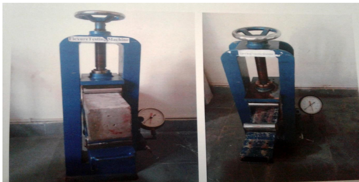
Figure 6.2 Test For Flexural Strength
