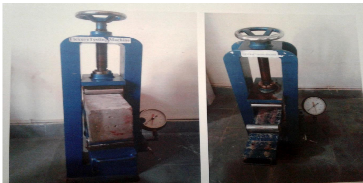
Figure 6.2 Test For Flexural Strength
