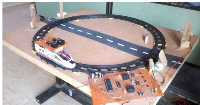
Fig 5.Gate control working train model
