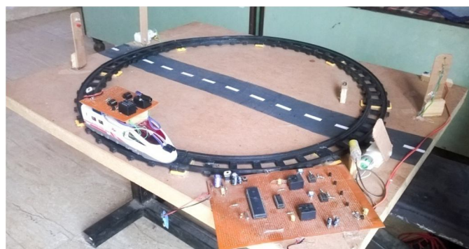
Fig 5.Gate control working train model
