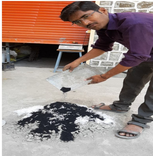
Fig(f): Addition of treated Crumb Rubber and Synthetic Fibre in concrete.
