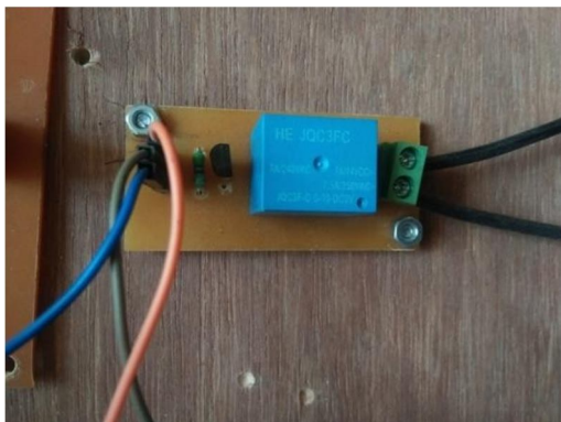
Fig no. 4.2a Model Relay circuit
