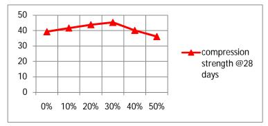
*E.* The above chart shows that from the metakaolin based recycled concrete aggregate with (0, 10, 20, 30, 40 and 50) percentage and their respective compression strength.
