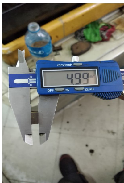
Fig. 4 Measuring W_a of machined workpiece on vernier calliper
