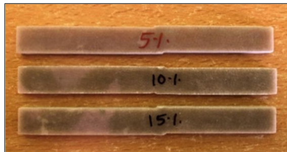
Fig. 8 Samples for Impact Test
