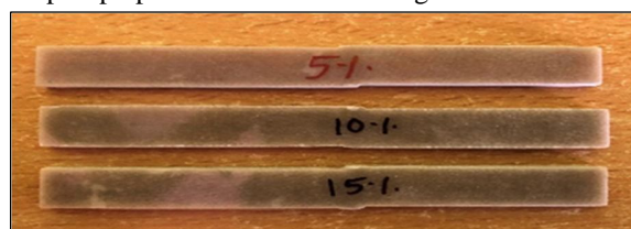
Fig. 6 Samples for flexural test
