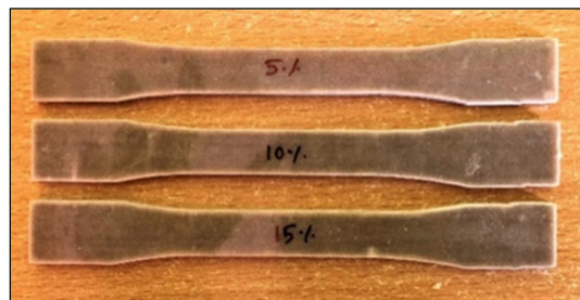
Fig. 5 Samples for Tensile Test
