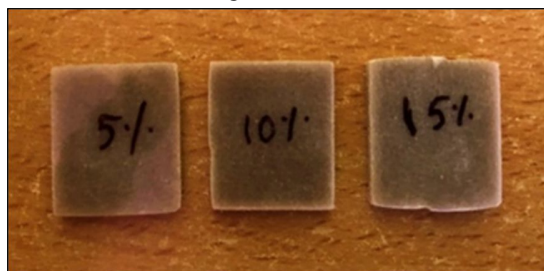
Fig. 9 Samples for Hardness Test
