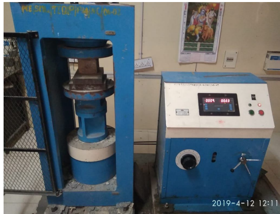
FIG 1 compressive strength test
