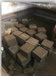
Fig. 2 Concrete Cubes in Curing Tank
