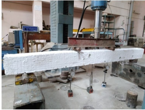
FIG 2 Experimental setup of the beam under two point loading
