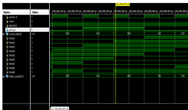
Figure 13: Simulation Waveform of 8-PSK Modulator at clock size 100us
