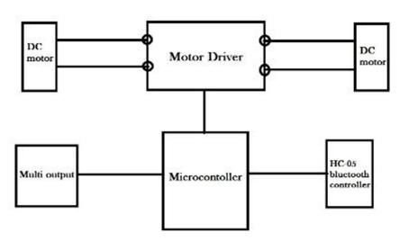
At first we connected both the DC motors with the L298N motor driver. Thereafter we connected the motor driver to the microcontroller Arduino UNO board. We take an HC 05 Bluetooth controller and connected with Arduino for wireless voice transmission. At last we used a multi output board for generating extra 5 volt power and connected with the Arduino.
