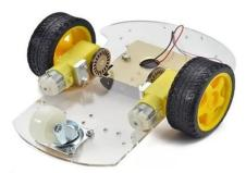
Chassis kit is probably the base of any moving project which will rotate in any angle if commanded. The frame, wheels, and machinery of motor vehicle on which the body is supported. The kit looks like the base of a car on which other components will be attached.
