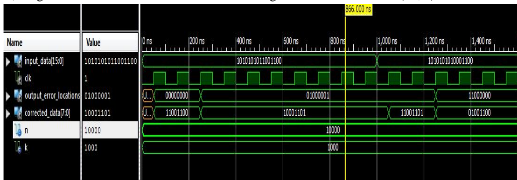
Fig. 3: Simulation Result of (16, 8) BCH code
