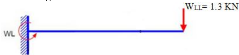
Fig. 3.6: Live load distribution on cantilever steps.
