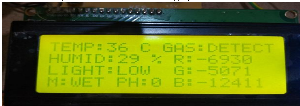
Fig 4: LCD display of Sensor Outputs
