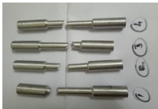
Fig3 Tensile Tested Samples
