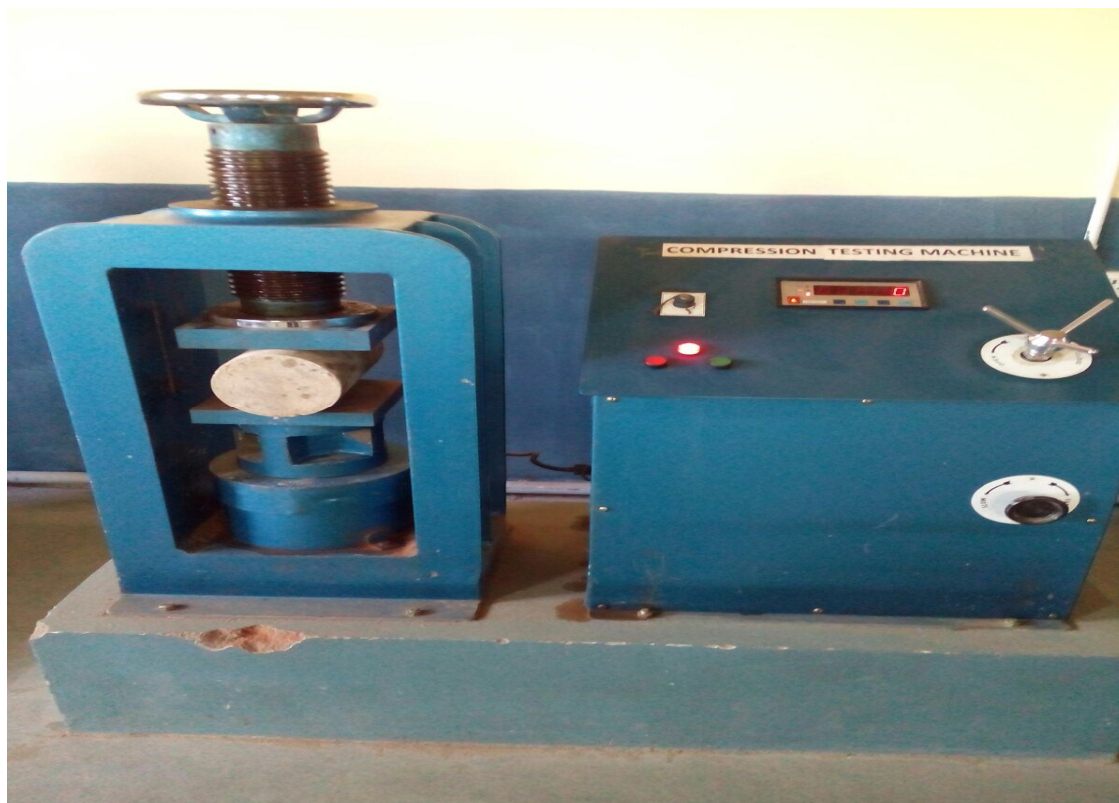
Figure 5.2 Split tensile strength of cylinder setup
