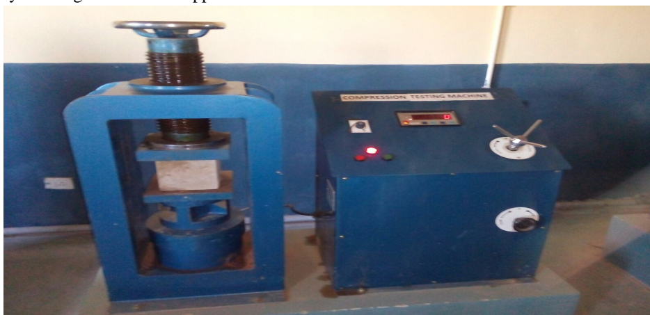
Fig. 5.1 Compressive strength of concrete cube setup
