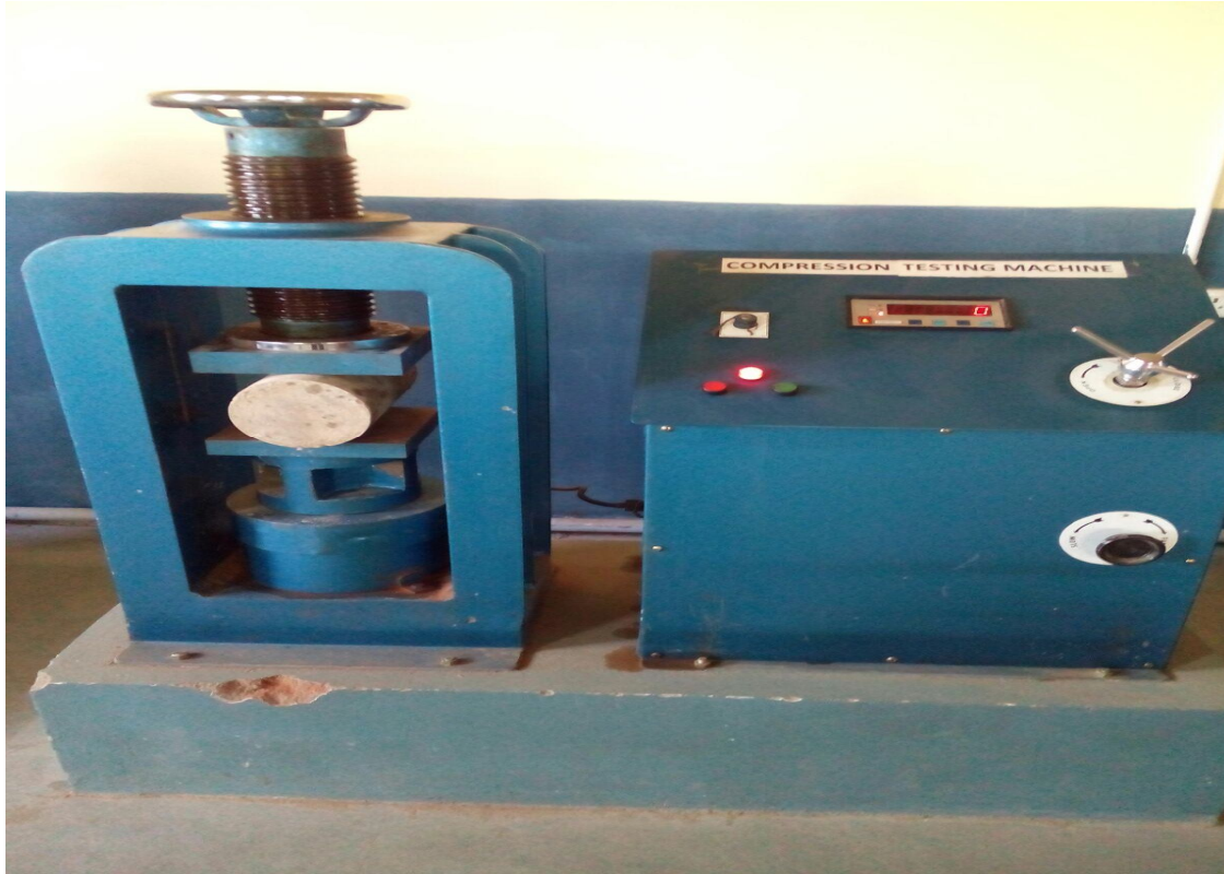
Figure 5.2 Split tensile strength of cylinder setup
