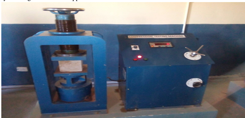
Fig. 5.1 Compressive strength of concrete cube setup
