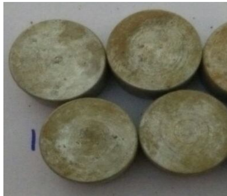
Fig 9 - Corrosion test samples (after 10days)
