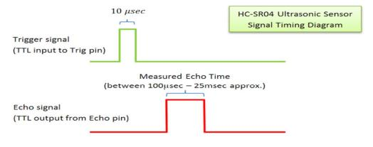
Distance (cm) = Measured Echo Time (in μsec)/58 Distance (inch) = Measured Echo Time (in μsec)/148
