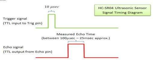
Distance (cm) = Measured Echo Time (in  $\mu$ sec)/58 Distance (inch) = Measured Echo Time (in  $\mu$ sec)/148
