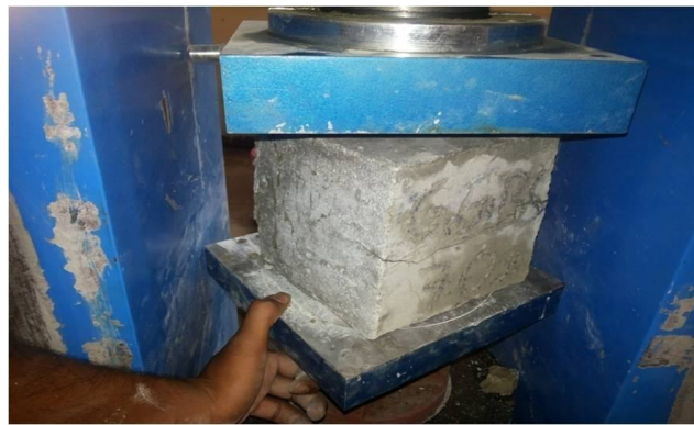
Figure 2 GGBS used Concrete under compressive test
