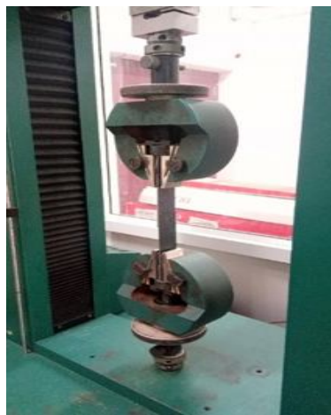
Fig 3.2 Tensile test conducting on Tinius Olsen machine
