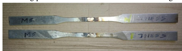
Figure: 2 dissimilar materials welded using TIG welding
