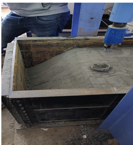
Fig. 3 Model tank for flat and slope cases including loading plate and dial gauges
