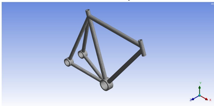
Fig. 3 Bike frame with meshing of 5mm
