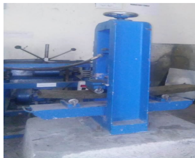
Testing of Flexural strength of slab
