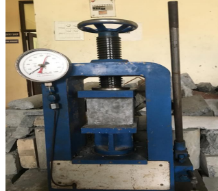
Compression test of cube
